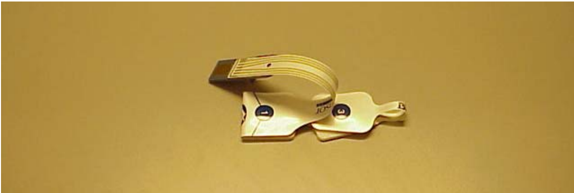
Figure 9-3 Connecting electrode #3 with #4, and #1 with #2.
